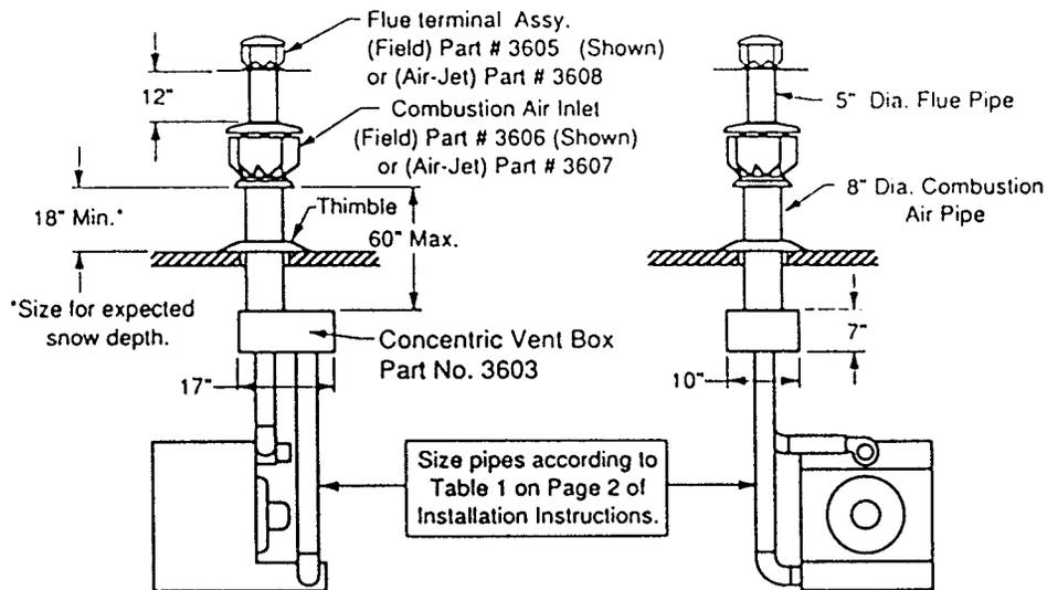
Figure 3. Vertical Concentric Venting
