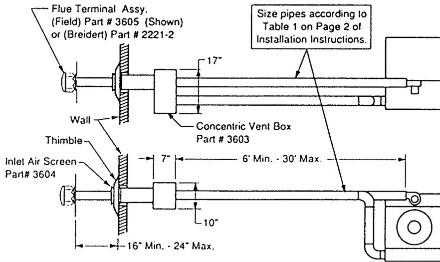
Figure 1. Horizontal Concentric Venting
