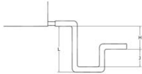
Drain pan trapping for section under negative pressure
