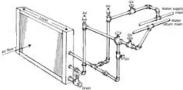
**Figure 11.** Typical piping for type 5A, 5W (2-row), D, DD, D1, D2, K, LL, OD, OK, OW, W3 (to 12-row), WA (2-row), WD, and WL water coils
