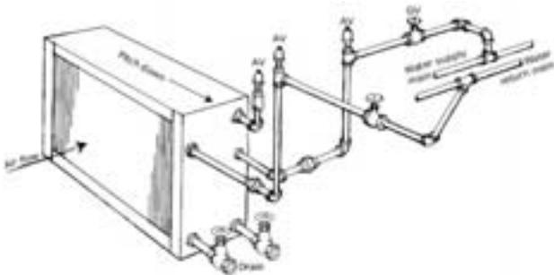
**Figure 12.** Typical piping for stacked water coils
