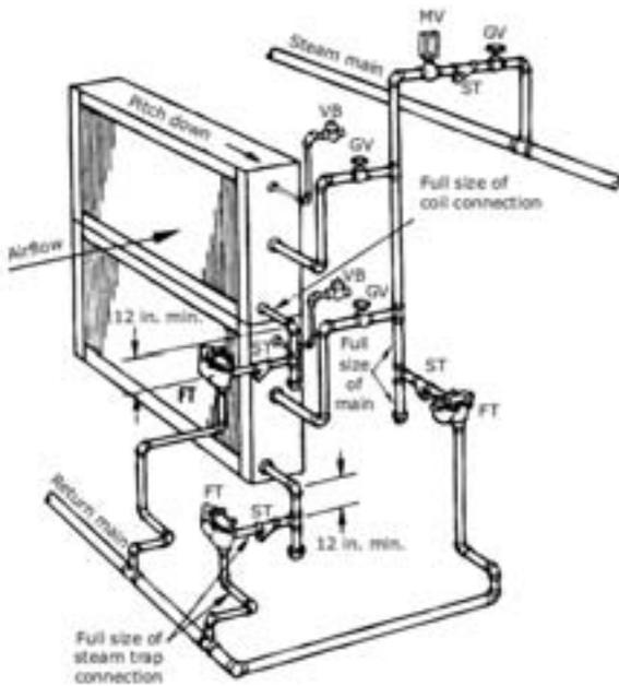
**Figure 6. Typical piping for type NS steam coils, vertical tubes for horizontal airflow**
