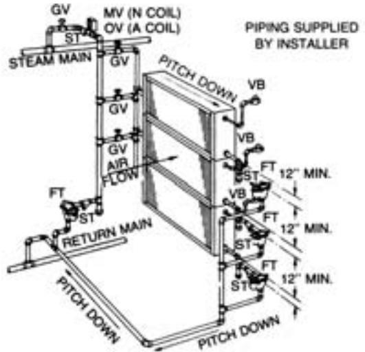
**Figure 8. Typical piping for type A or N steam coils, vertical tubes for horizontal airflow**
