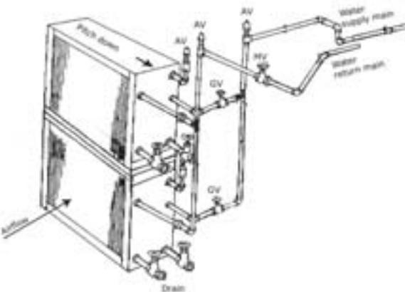
**Figure 13.** Type T and ST water coil
