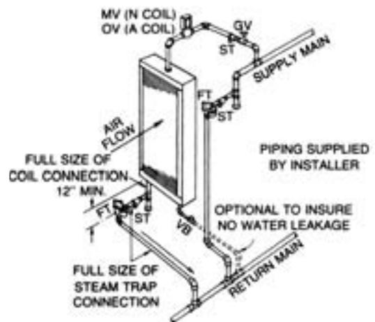
**Figure 9. Typical piping for type T steam coils, horizontal tubes for horizontal airflow**
