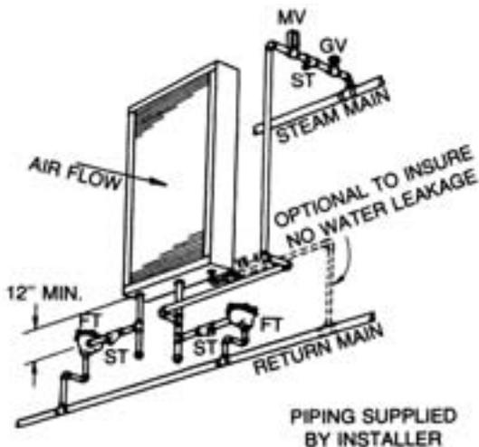
**Figure 7. Typical piping for type A or N steam coils, horizontal tubes for horizontal airflow**
