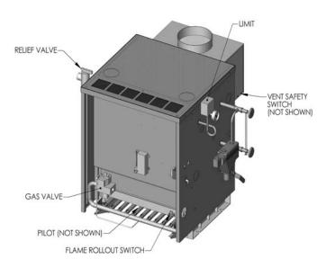
1a. Limit (Steam Boiler). An electrical device that automatically interrupts the boiler operation when the steam pressure exceeds the "CUT IN" pressure plus the differential (1 to 5 psi). Maximum Pressure setting is 14 psig. The set point is usually less than 5 psig.
