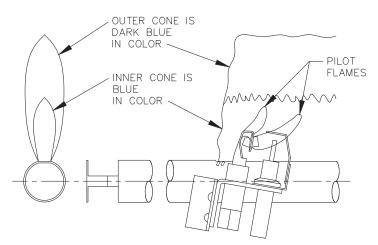
Figure 6: Intermittent Ignition Pilot Configuration and Flames
