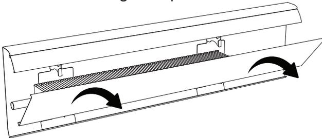
3. Remove any existing damper sections.
