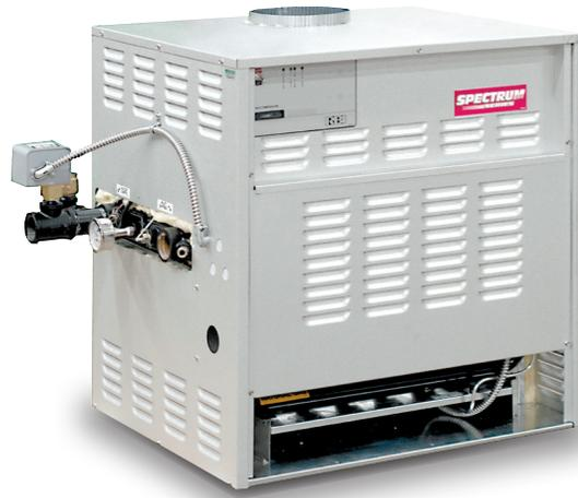
All Spectrum units come standard with Galvalume jacketry. Galvalume is a coating consisting of zinc, aluminum and silicon used to protect metal from oxidation. Galvalume is applied to a material (steel) using a continuous hot-dipping process, which creates up to 1ML protective barrier against rust and oxidation.
