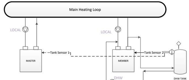
Ensure that the Member boiler's Damper and System pump control are configured correctly with the assumption that the Master is not powered. Also ensure that any other System settings related to outside air temperature sensing and system interlocks are set to provide safe operation.
