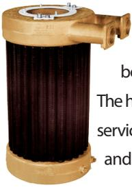
or cast iron headers – standard on all Futera II boilers. The tubes are individually field replaceable. The heat exchanger is superior in design, durability and serviceability – each is hydrostatically tested, approved and stamped for 160 psi ASME operation.
