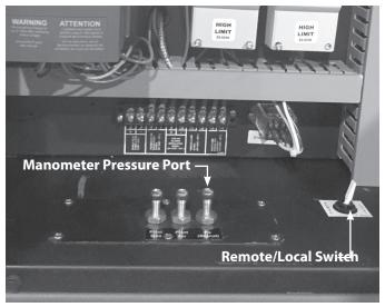
c. Set pilot gas pressure to 3.0 in WC ( $\pm 0.5$  in) by adjusting the pilot gas pressure regulator, inside the air box. Access from the boiler top cover. See Figure 17.
