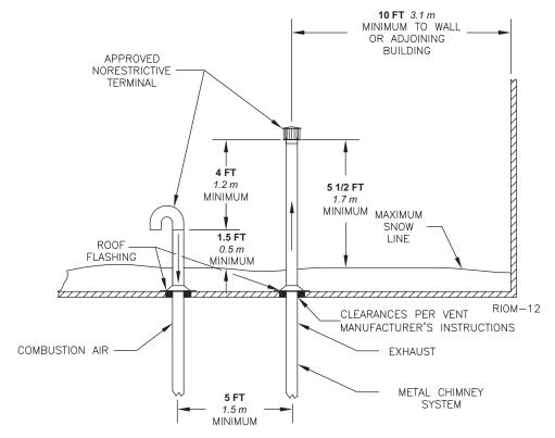
Figure 4 Horizontal Air Intake and Venting for Multiple Direct Vent Systems
