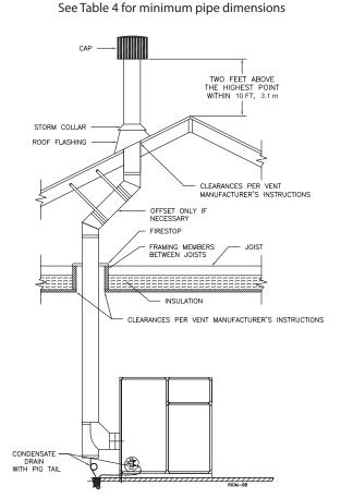
Vertical Venting with a Metal Chimney System
