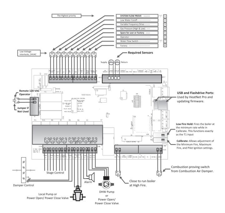
Figure 19 RBI Field Wiring to HeatNet Board (Board Revision 3.0 and Greater)
