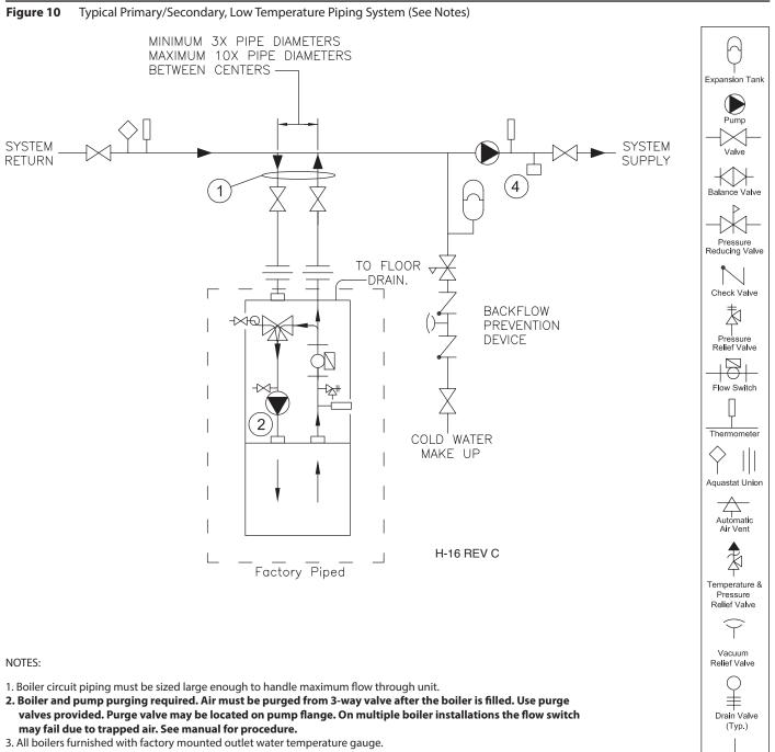
4. For HeatNet operation, a sensor is required and installed at a minimum of 12 inches from the primary tee.
