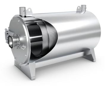
Hydroforming insures a uniform and consistent gap between the tubes facilitating consistent exhaust gas circulation and uniform heat transfer throughout the entire heat exchanger.
