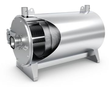
Hydroforming insures a uniform and consistent gap between the tubes facilitating consistent exhaust gas circulation and uniform heat transfer throughout the entire heat exchanger.
