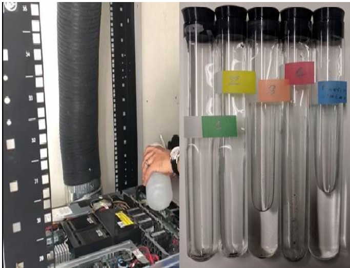
Figure 7: COLLECTED DUST SAMPLES FROM SERVER CHASSIS
