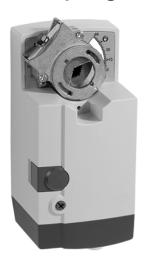
These direct-coupled damper actuators provide adjustable modulating control for: air dampers, VAV units, air handling units, ventilation flaps, louvers, and reliable control for air damper applications with up to 4.6 m2/50 sq ft (seal-less dampers; air friction-dependent).
