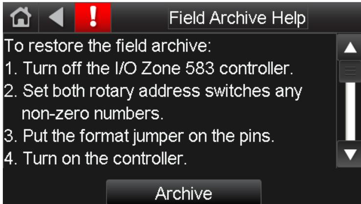
5. Run and Error LEDs cycle 3 times opposite of each other, then return to normal operation once the process is complete. The Run LED flashes once per second during normal operation.
