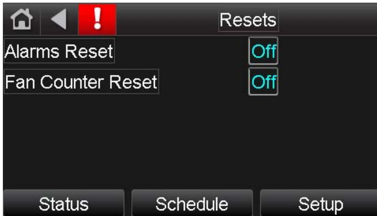
If the Alarms Reset setpoint was left in the “On” state continuously, the alarms can still trigger on alarm conditions. However, to reset the alarms from this state you must change the Alarm Reset parameter to “Off”, then “On”, then “Off” again. Otherwise, the alarms will not reset and you will not be alerted if an alarm that was previously triggered happens to trigger again during the period the initial alarm remained active.
