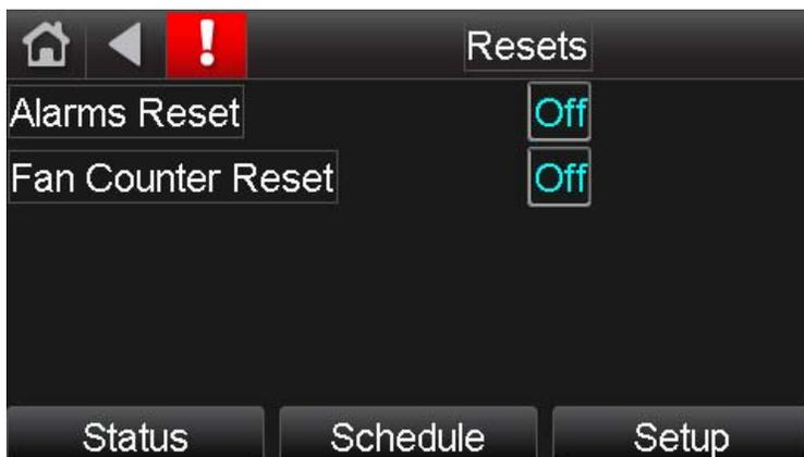
This section will assist the user in resetting alarms and the fan cycle runtime counter, which have been displayed on the *Equipment Touch*.
