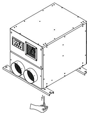
Figure 5 - hanging assembly attachment.
