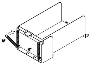
**Figure 12 – The process of spring replacement**
