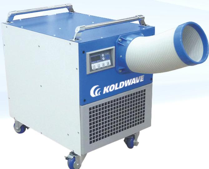
The unit automatically dehumidifies (dries and cools) the air then reheats the air to a room neutral condition. With a moisture removal capability of 120 Pints/Day based on AHAM Rated Conditions of (80F DB/60%RH). Permanent, cleanable filters are provided for both the condenser and evaporator intake. An internal condensate reservoir and pump remove the collected water and disperses it through a 30' long condensate line to the nearest drain.
