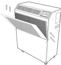
**Figure 6 – Removing Filters**
