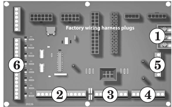
**Figure 12** 120VAC power service terminals on electrical connection board — See Figure 15 for location of the power terminal strip
