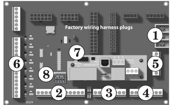
**Figure 2** 120VAC power service terminals on electrical connection board — See Figure 15 for location of the power terminal strip
