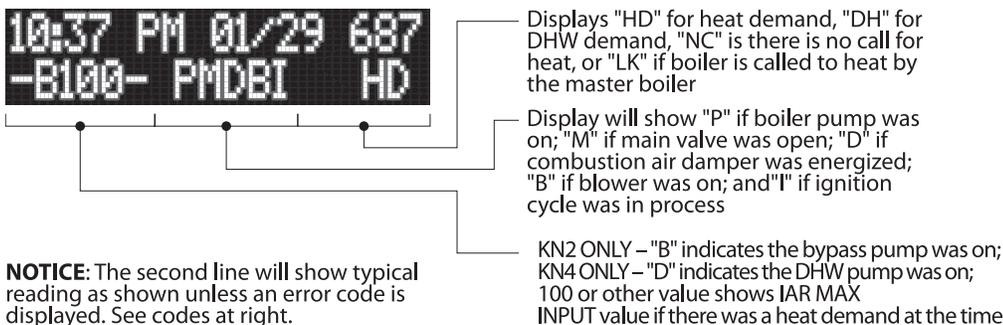
**NOTICE:** The second line will show typical reading as shown unless an error code is displayed. See codes at right.
