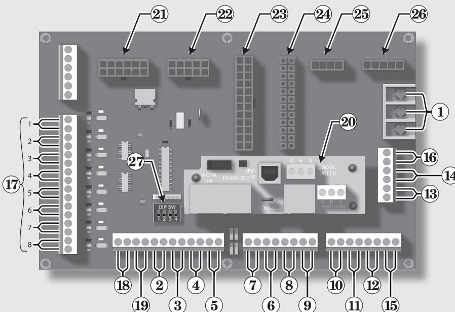
(All boiler wiring is made with non-interchangeable plug-in harnesses, connected to this board)
