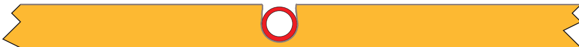
FIGURE A-1, a cross section, showing PEX pipe in groove and board with aluminum top layer
