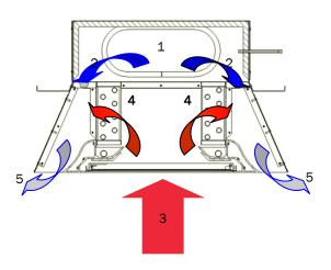
Primary air (1) is introduced into the Active Chilled Beam through a series of nozzles (2). Due to the fluid dynamic properties of nozzles, room air (3) is drawn into the Active Chilled Beam through a secondary water coil (4) by an induction process.
