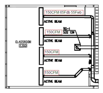
Each unit requires supply and return connections for 10.0 gpm, 56°F chilled water.
