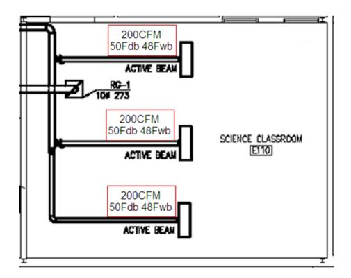
Each unit requires supply and return connections for 3.0gpm, 56°F chilled water.
