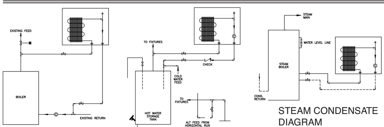
On a typical forced hot water system, connect return to inlet side of circulator and supply upstream of remotely operated valve. Unit may also be connected to mains of an existing loop system of sufficient capacity. Operation will be influenced by the system circulator and associated controls.
