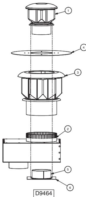
**Figure 1b – 6 Inch Combustion Air Inlet Kit**
