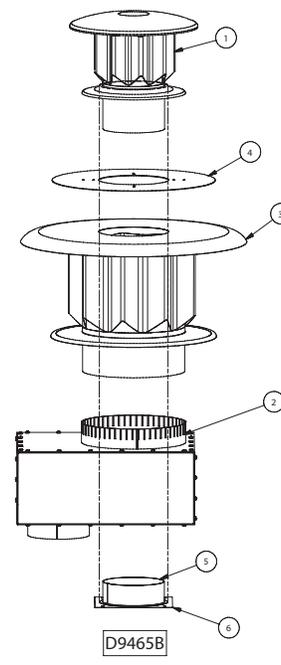
\*Deflector Disk comes with brackets and screws for installation.
