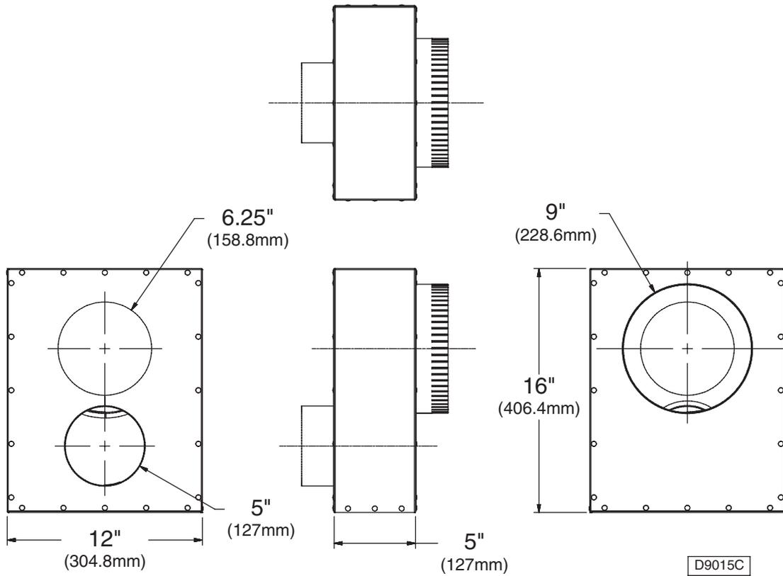
Figure 2b – 6 Inch Combustion Air Inlet Box Assembly
