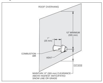
Figure 17 - Horizontal Sidewall Concentric Venting, Multiple Unit Vertical Layout
