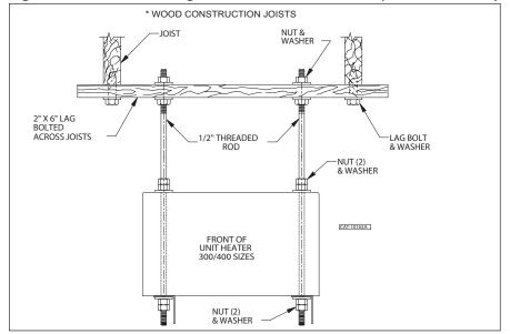
\*Note: Angle mounting brackets are provided by the manufacturer for unit sizes 300/400. All other hanging hardware and wood is not included with the unit and should be field supplied.
