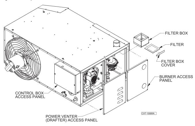
Figure 27 - Flue Collector/Drafter Assembly
