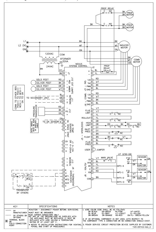
Figure 7D – Unit Wiring Diagram, High Efficiency Unit Heater Size 300/400, Equipped with Natural or Propane (LP) Gas, Modulating with Outside Air Reset (Master)
