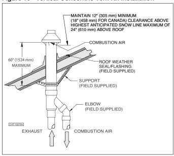
Figure 20- Vertical Concentric Venting, Roof Termination
