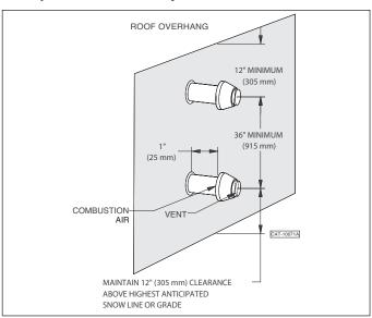
Figure 18 - Horizontal Sidewall Concentric Venting, Multiple Unit Horizontal Layout
