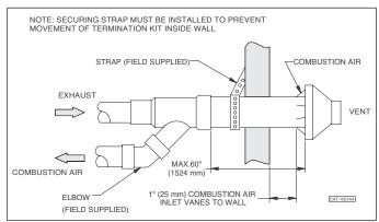
Figure 16 - Horizontal Sidewall Concentric Venting, Single Termination
