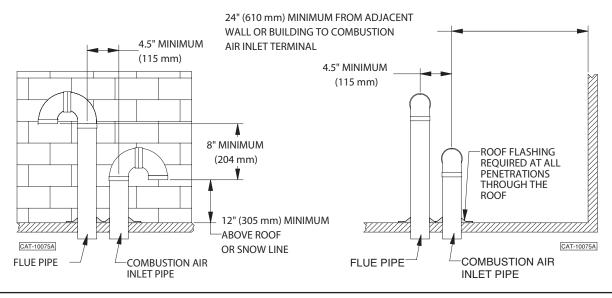
Figure 12 - Vertical Two Pipe Separated Combustion Venting, Sloped Roof Termination
