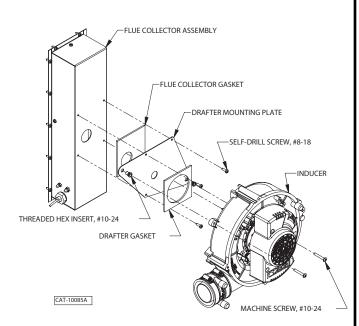
Figure 28 - Air Gas Inlet Assembly
