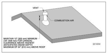
NOTE: Keep assembly free of insulation during installation.
