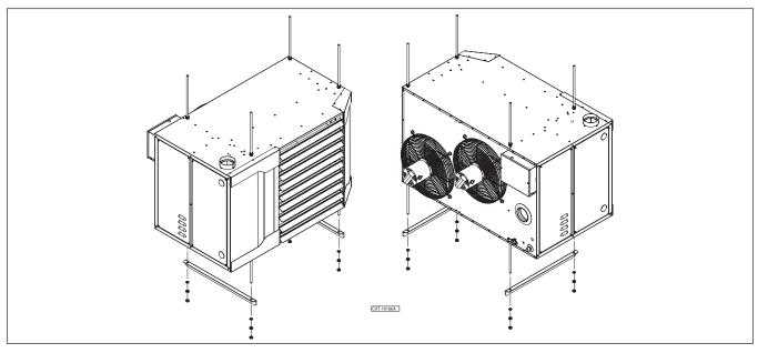
Figure 3C - Heater Mounting: Steel Construction (for all sizes)
