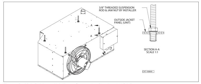
Figure 3B - High Efficiency Unit Heater Suspension (for sizes 300/400)
