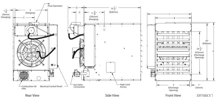
$<sup>^{\</sup>star}$  Flue collar is factory supplied with unit; to be field installed per included instructions.
