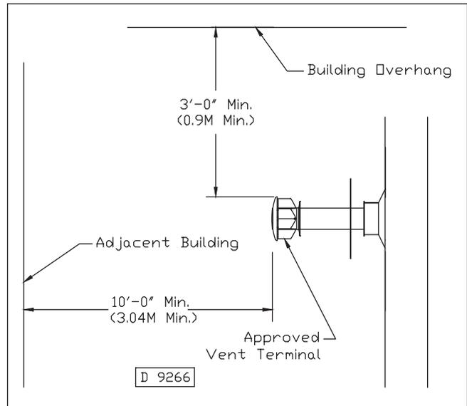
**Figure 5 - Horizontal Vent Termination**
