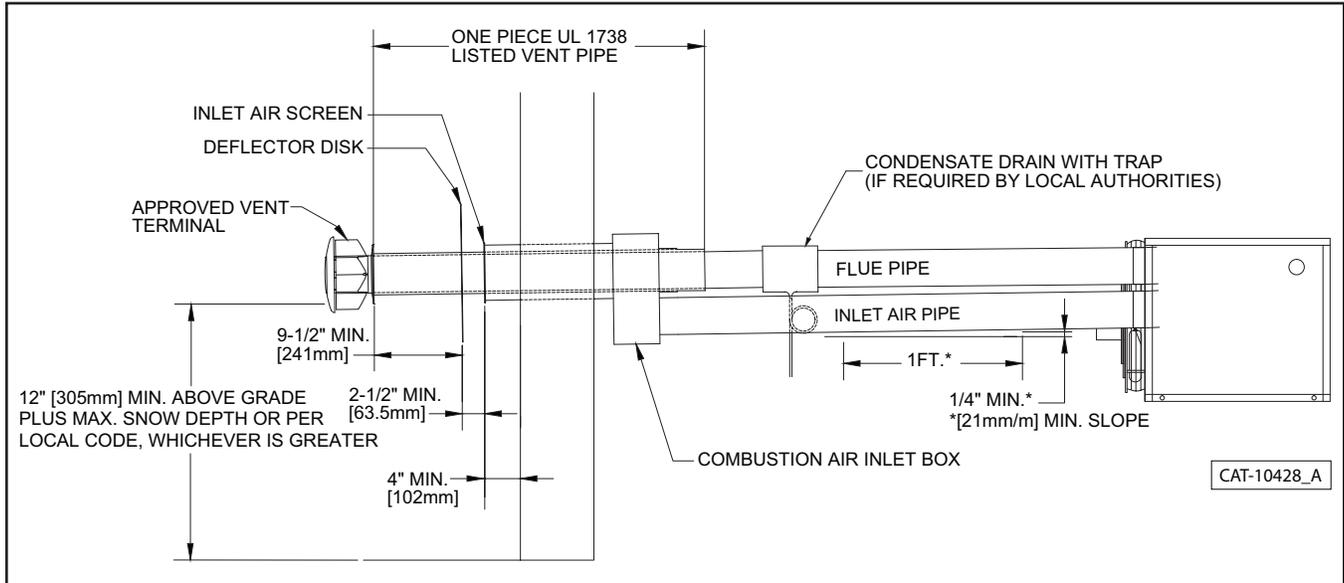
**▲ WARNING** Never use pipe other than 5 inch diameter. Never use PVC, ABS or any other nonmetallic pipe for venting! To do so may result in serious damage to the unit and or severe personal injury or death!
