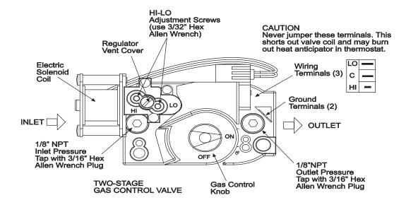
This appliance is equipped with a step-opening, combination gas valve. The maximum supply pressure to the appliance is 14" W.C. or 1/2 P.S.I. If the line pressure is more than the maximum supply pressure, then a second stage regulator, which corresponds to the supply pressure, must be used.
