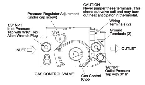
This appliance is equipped with a step-opening, combination gas valve. The maximum supply pressure to the appliance is 14" W.C. or 1/2 P.S.I. If the line pressure is more than the maximum supply pressure, then a second stage regulator, which corresponds to the supply pressure, must be used.
