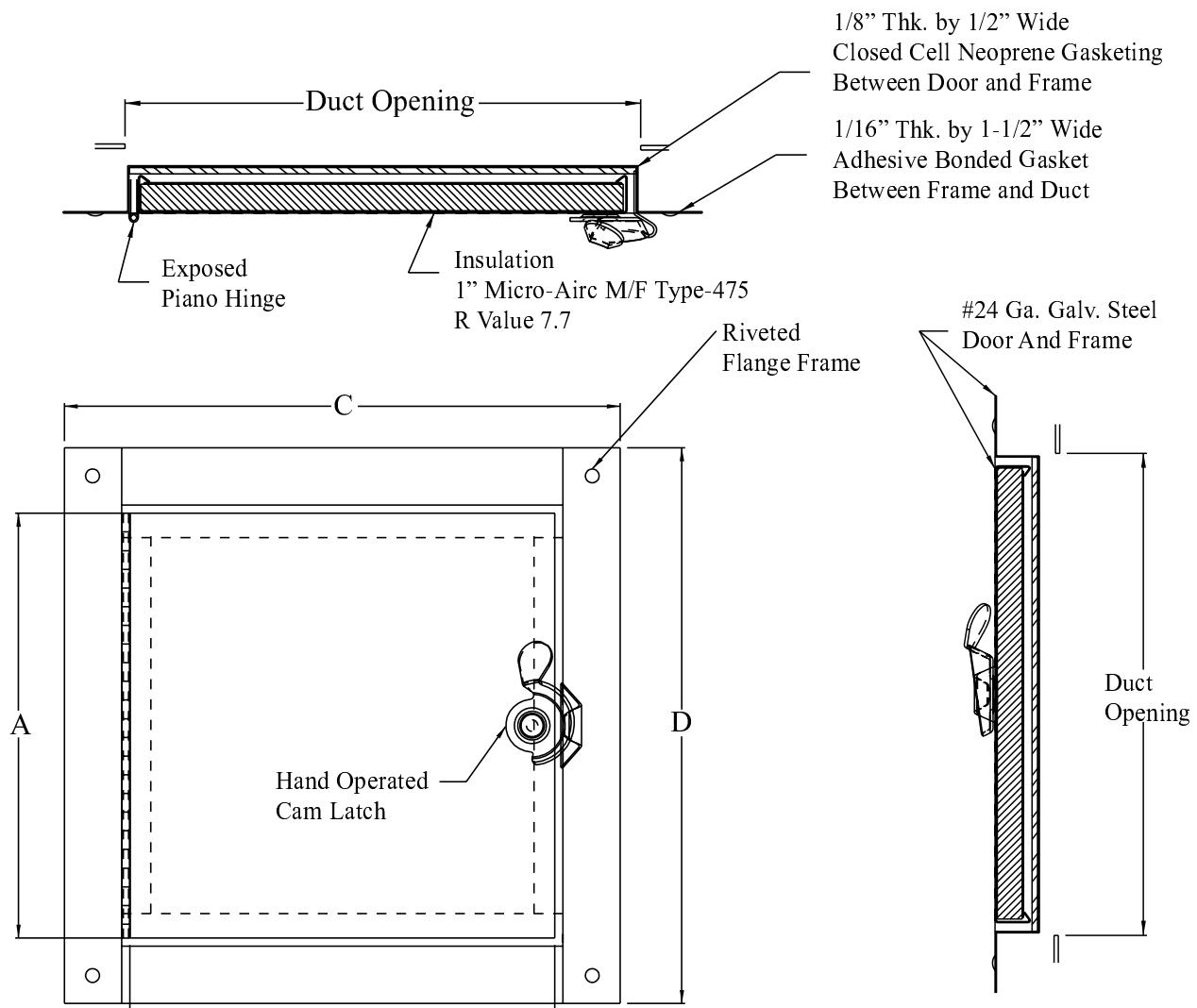
**Standard Features:** Piano Hinged Door Panel, Self Tightening Hand Operated Cam Latch, Galvanized Steel, Mill Finish
