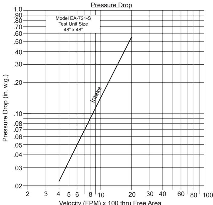
Intake air converted to standard air density.
