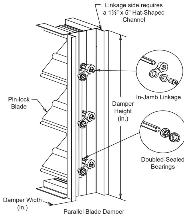
**Extruded Aluminum Damper • 5" Deep • 6" Single Thickness Blades • Parallel (506) or Opposed (507)**
