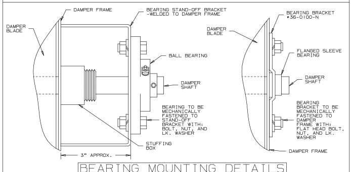
BEARING STAND-OFF BRACKET IS TYPICALLY USED WHEN FURNISHING A STUFFING BOX.
