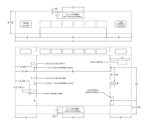
Left hand piping connections shown, right hand opposite. Piping hand determined when facing air outlet. Electric junction box location may vary depending on control requirements. Contact Factory.
