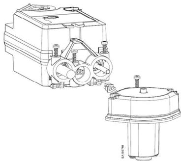
Figure 2. The EFL and OpenAir Fire and Smoke Damper Actuator.
