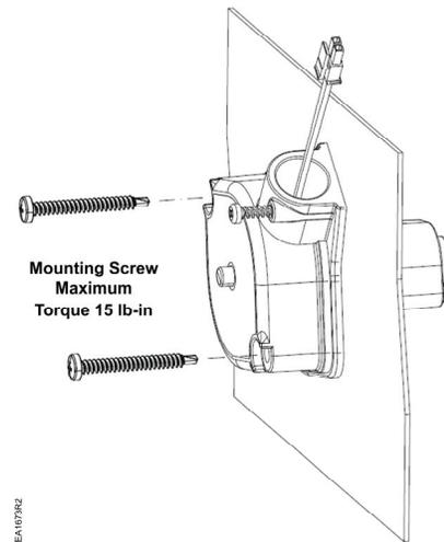
Figure 5. Providing Proper Sensor Temperature Detection Access.
