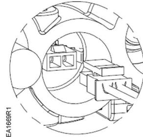
Figure 3. Proper Clip Positioning.
